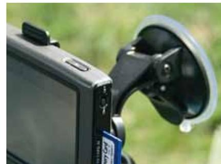
*The suction cup worked well in our test. The SD card stores field boundaries and area covered in kml format. Once imported to the office PC, data are mapped out in Google Earth.*
