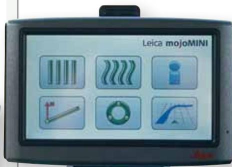
*Available field guidance features are A-B, contour, A+ heading and pivot. The button down to the right activates boundary recording which includes field size computation.*
