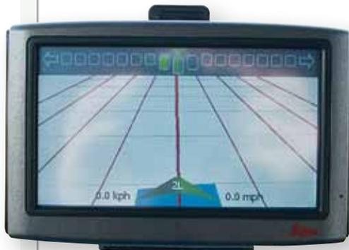
*The system combines lightbar guidance (at the top of the screen) with perspective view lines to make up for the small screen. The concept proved very effective and was indeed a great help for steering.*
