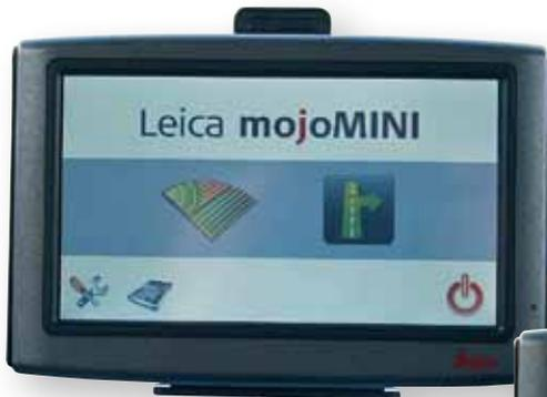
After booting the system, users either press the parallel guidance or street navigation icons which appear on the start-up screen. Parallel guidance is the left icon. In addition, they can also choose to have a calculator or setup icon displayed in the bottom left corner of the screen.
