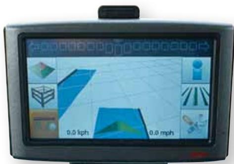
*mojoMini also records area covered. In addition, the operator can select the left or right border to compute the area within the boundary. Photos: Böhrnsen, Holtmann*
