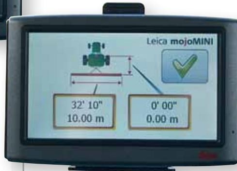
*Work width and distance from the antenna to the implement need to be verified before you can start a job. Units are displayed in imperial and metric units. There is no option to select either.*
