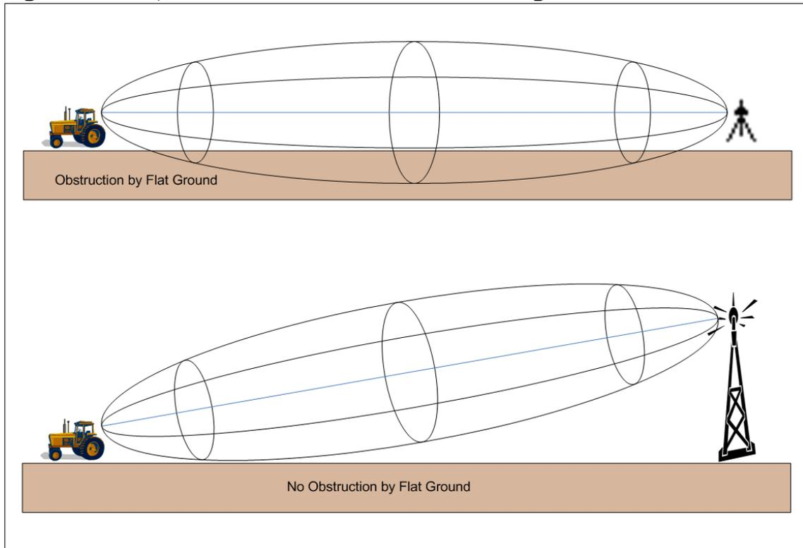
*Note: it is possible to have too much clearance as the radio reflections in the second Fresnel zone interfere with each other in a way which reduces the signal at the receiver. However, when setting up the base radio on a tower it is unlikely that you will get the base antenna high enough to suffer this problem.*
