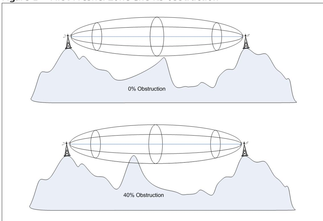
Figure 1 shows two radio towers communicating with each other in two situations. The first situation shows no obstruction of the first Fresnel zone and the second shows some obstruction of the first zone.
