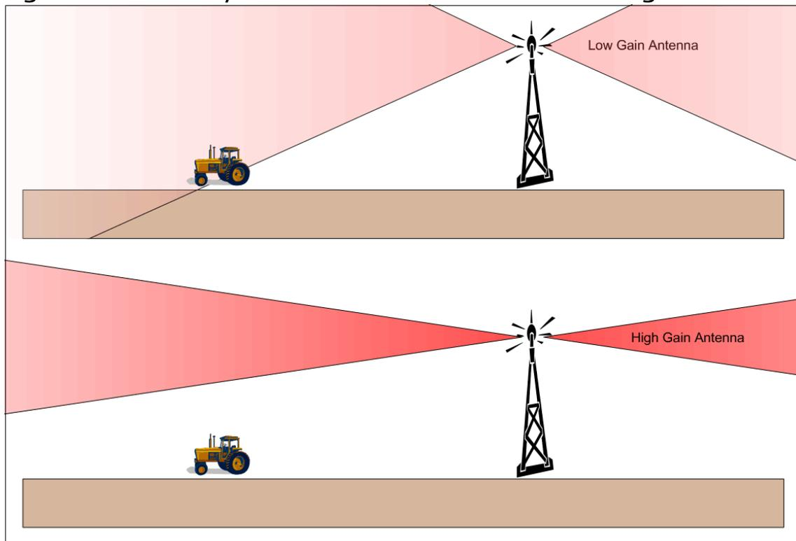
**NOTE:** although the high gain antenna pushes a stronger signal further out it may cause problems when trying to receive the signal when you are too close to the antenna and it is mounted high up a tower. Also note that the diagram may exaggerate the reduction in transmission area and was drawn only to explain the concept.
