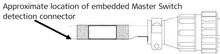
Figure 3: Embedded Master Switch Detection Connector
