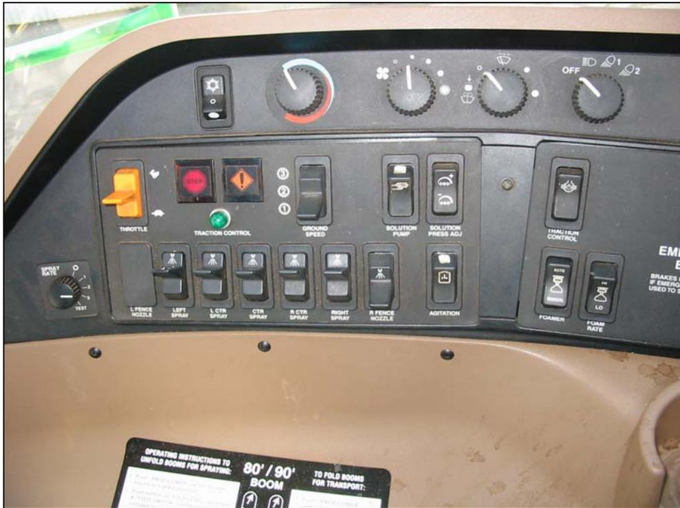
**Figure 2.2 John Deere Section Switch Panel**
